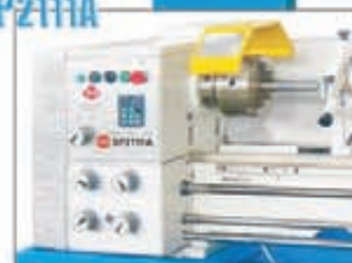
Variable speed gear head lathe with DRCD other specifications are the same as SP2111
