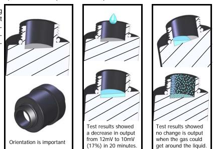
**Shock:** Dropping a sensor that has been removed from its shipping package can damage the sensor in a number of ways: (a) compromise electrical connections resulting in erratic readings, (b) broken wires, (c) dislodging an anode which contacts the a cathode connection creating a short circuit, (c) tests show that dropping a sensor from 3 ft. onto a carpeted concrete office slab results in a reduction in signal output ranging from 25% to zero signal output.
